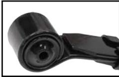
**Mid Eye** - Adding a counter bend at the base of each eye repositions the mounting bolts to sit along the centerline of the spring stack. This brings the axle closer to the chassis, lowering the vehicle roughly half the diameter of the spring eyes, or approximately 1".
