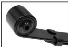
**Standard Eye** - OEM leaf springs position the eyes above the centerline of the spring stack. This places the axle at its furthest distance from the chassis, commonly referred to as the stock ride-height position.
