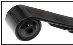
**Reverse Eye** - Coiling the spring eyes in the opposite direction from stock, places the mounting bolts below spring-stack centerline, resulting in a ride height roughly 1-1/2" below stock. The ultra-low stance creates a sleek vehicle profile, and lowers the vehicle's center-of-gravity for improved handling.
