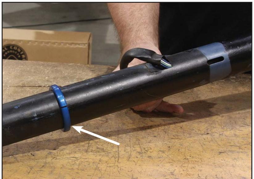
16. Insert the replacement steering shaft into the column tube.
