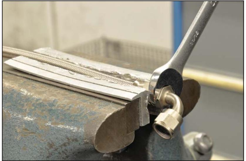
17. The fitting is assembled and we have lined up the tube of the fitting to a index mark. This is an important step because the fitting can not be rotated once they are tight.
