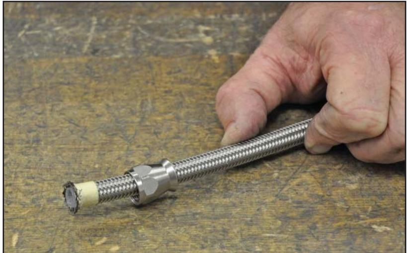
8. Place the brass ferrule in between the Teflon hose and steel braid as shown.
