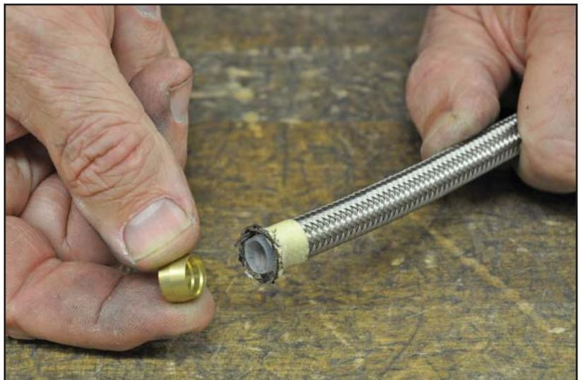
9. Apply pressure against the ferrule until the Teflon hose is seated against the inside lip of the ferrule.
