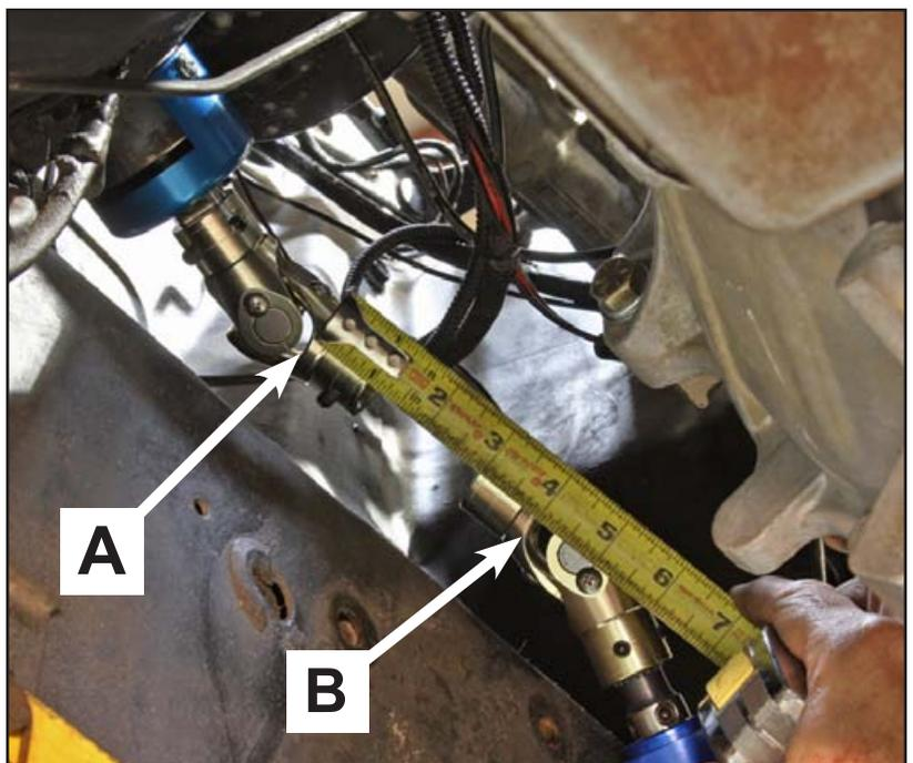
10. Place supplied intermediate steering shaft into a vise and cut square to the determined length.
