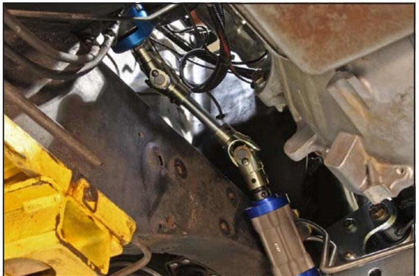
17. Move the steering wheel through its complete travel. There should be any binding. If bind is detected in the steering wheel you may need to shorten the 3/4-DD shaft until the steering moves freely.
