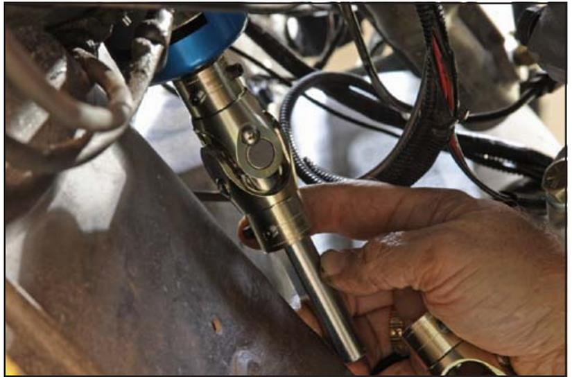
15. Insert the shaft into the lower u-joint.
