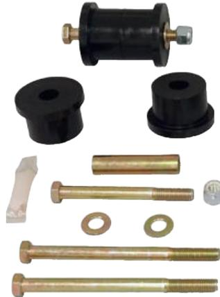
**Description:** Polyurethane bushing set, includes bushings, sleeves, mounting hardware, and poly lube. Fits 2"-bore x 2-1/2"-wide front leaf-spring eye with 1/2" mounting bolt. Directly replaces RB82 rubber bushing.
