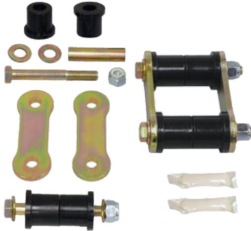
**Description:** Shackle set includes scalloped shackle plates, urethane bushings, sleeves, hardware, and poly lube. Fits 1-3/8"-bore x 2-1/2"-wide rear leaf-spring eye and chassis mount, uses 1/2" mounting bolt.
