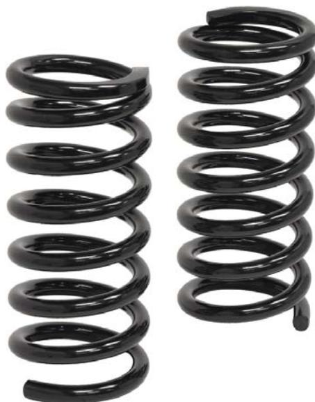
**Description:** 1" lowering front coil-springs (560 lb/in), 12-1/8" free length, ground top end with open bottom end, black powder-coat finish.
