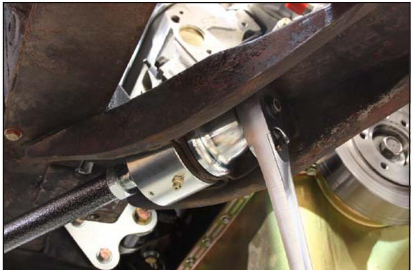
18. Apply Loctite™ threadlocker to the 3/8” button-head screw, and then install with a flat washer and lock washer.
