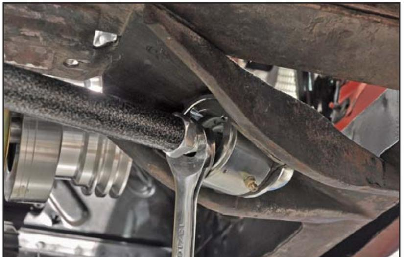
23. Once adjustment is complete, tighten the jam nut against the strut rod. Hold the pivot stud hex with a wrench to prevent from adjusting the strut rod length.
