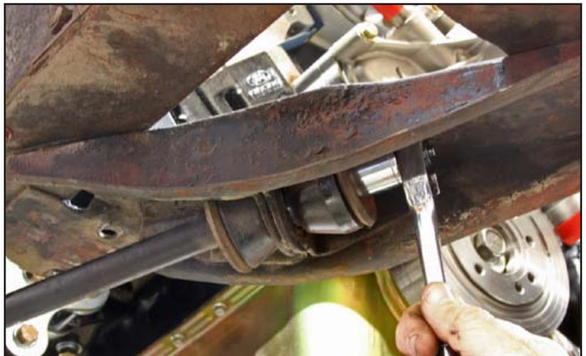
8. Remove the steel sleeve from the frame mount with a chisel.
