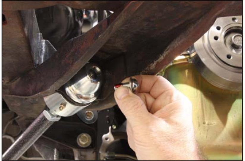
20. Loosely bolt the strut-rod plate to the lower control arm using hardware shown.
