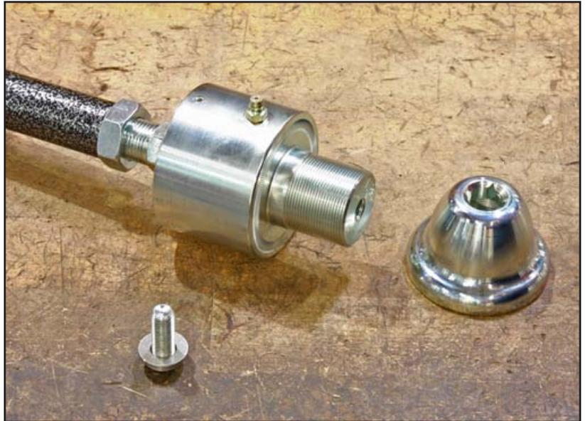
14. Rest the strut rod plate on top of the lower control arm before inserting the pivot housing into the factory frame mount.
