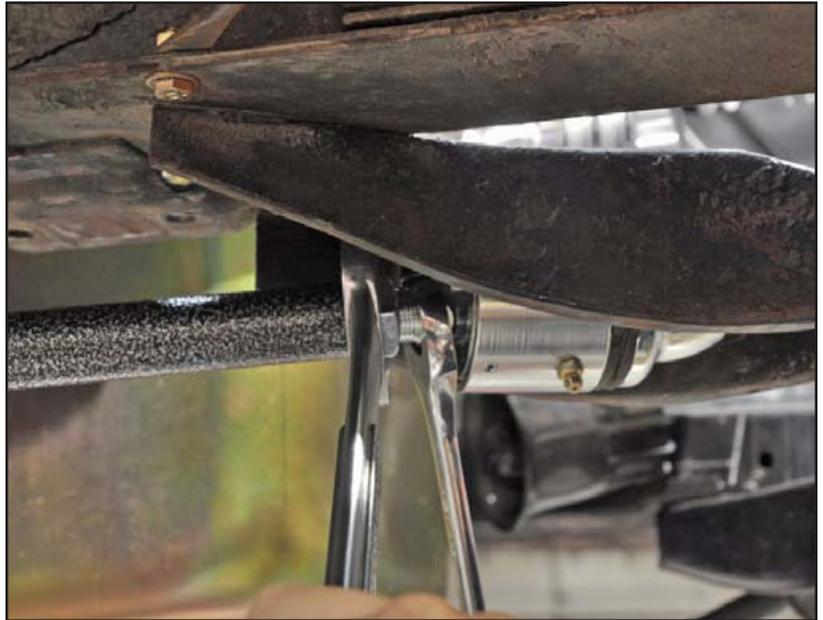
24. Tighten the socket-head cap screws to 60 lb-ft.
