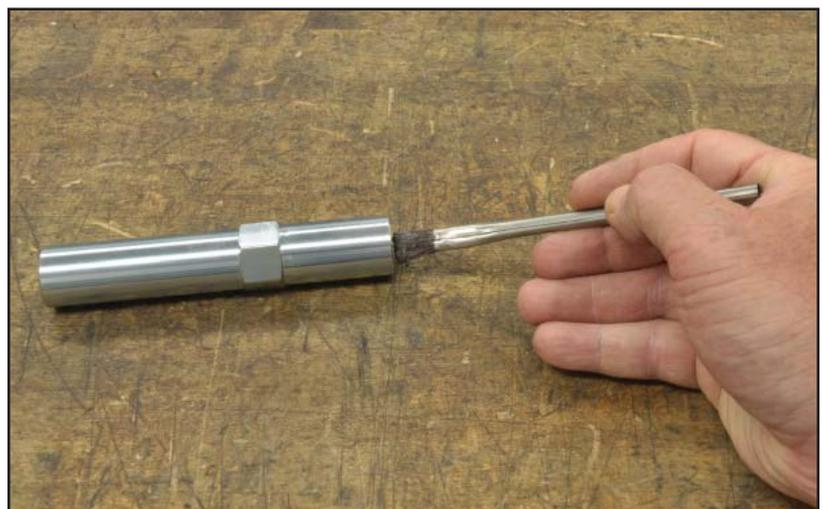
5. Thread a right hand jam nut (3102-069-18RC, clear zinc) onto each outer rod end until 1" of threads are past the nut.
