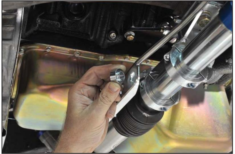
12. Insert the inner tie rod into the adapter.
