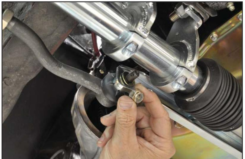
14. Tighten the locknut with a 5/8" wrench. You will have to push the tie rod into the tapered adapter while tightening the locknut.
