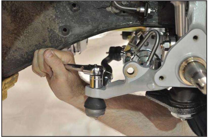
18. Insert the cotter pin through the castle nut and bend the one leg over the tie rod end and the second around the castle nut.
