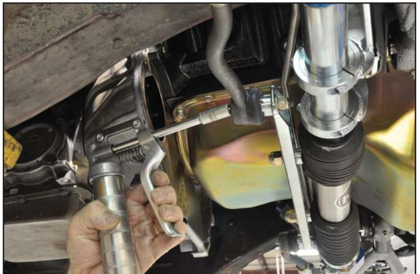
20. Once you have the front end aligned tighten the jam nuts against the adjuster.
