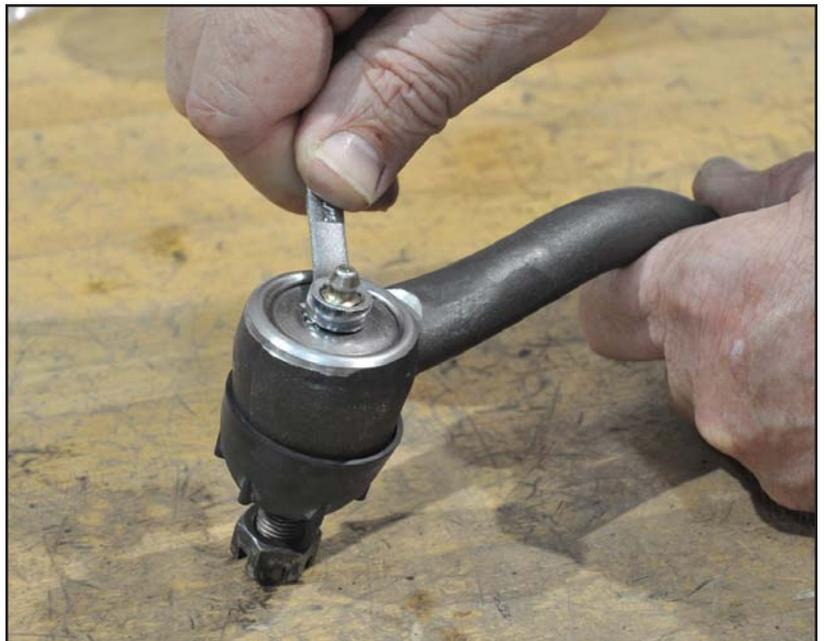
11. Insert the tapered adapter into the end hole of the rack's center link or factory drag link.
