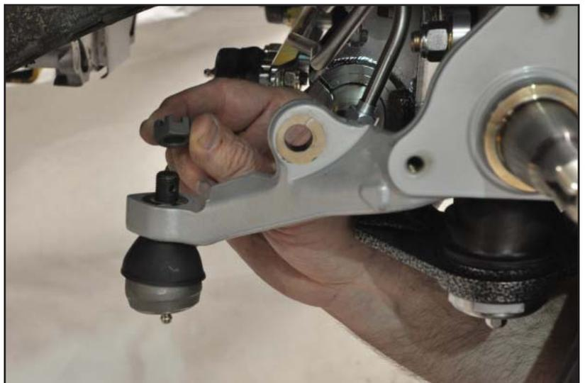
17. Tighten to 40 lb-ft. Then align the cross-hole with a slot in the castle nut, by tighten not loosening the castle nut.
