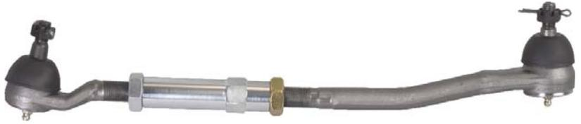
9. The assembly should be the same length as the OEM one removed, if not turn the adjuster to correct the length.
