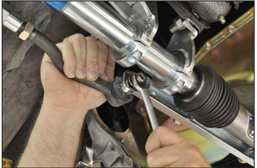
15. Align the outer tie rod with the steering arm on the spindle and insert it into the tapered hole as shown.
