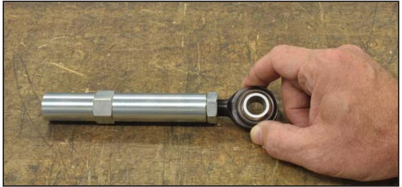
13. Thread the left hand jam nut (3102-69-18LY) (yellow zinc) onto the inner tie rod to end of the threads.
