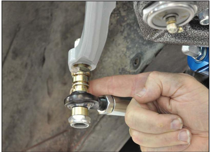
22. Thread the 5/8-18 jam nut onto the stud to temporarily secure shim stack and rod end during the measurement procedure. The jam nut should be snug to prevent any free play of the shims during bump steer setup. The jam nut will be replaced by a locknut after final adjustment. If the vehicle will be moved before final adjustment install locknuts in place of the jam nuts for safety purposes.
