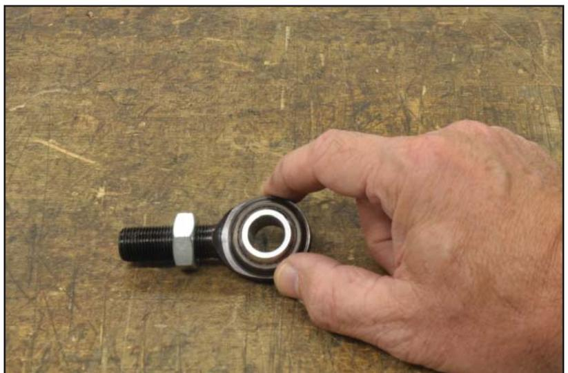
11. Screw the rod ends (3136-063X063-R) into the billet adjusting sleeves until the jam nut contacts the sleeve. The hex on the billet sleeve is closest to the left-hand threads.
