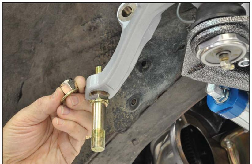
20. To begin setting up the shim stack, place the largest adjustment shim (3/8") onto the stud.
