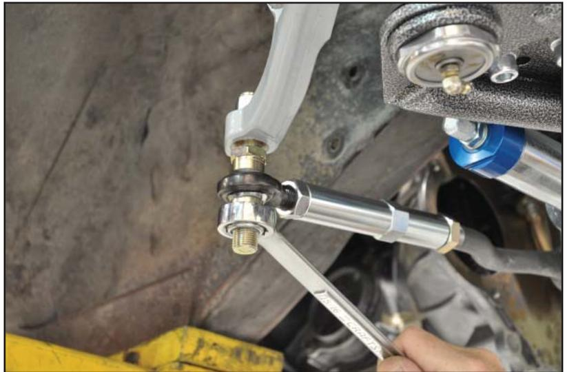
***Springs must be removed from suspension system before proceeding.***
