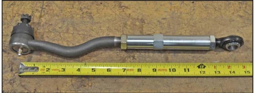
18. Install tapered stud (7900-227-B) (7/8" hex) into steering arm and secure with 7/16" washer (3120-044S-Y) and 7/16-20 locknut (3131-044-20Y) (5/8" hex).
