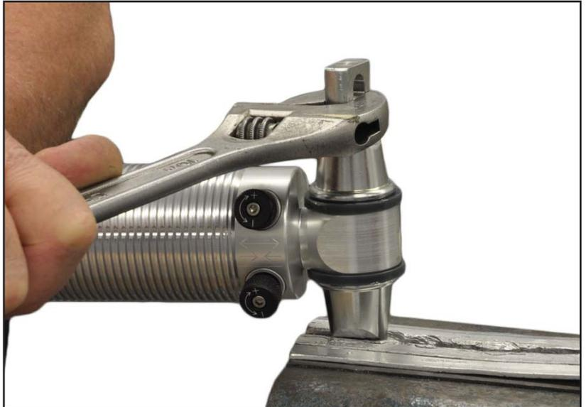
9. **CLOCKING STEP:** Tighten the assembly to the very first evenly-clocked position (less than one-half turn). Bring the crossbar into position in small increments and verify its position at each step; clocking it in one motion risks overtightening. A straightedge should be placed against the exposed crossbar tab to tell if the tab is inline with the vice jaws.
