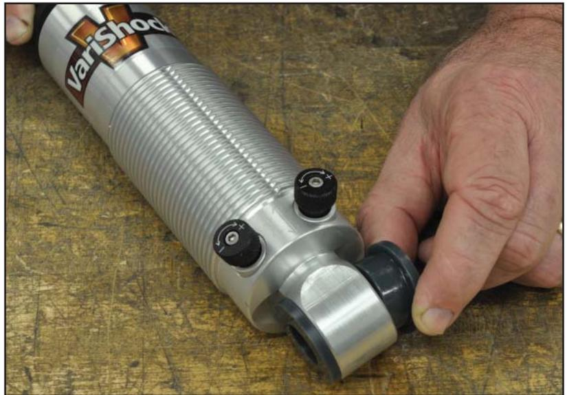
2. Press two bushings into each shock eye.
