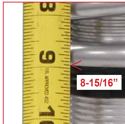
Measure the bottom end of the spring.
