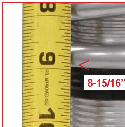
Measure the bottom end of the spring.
