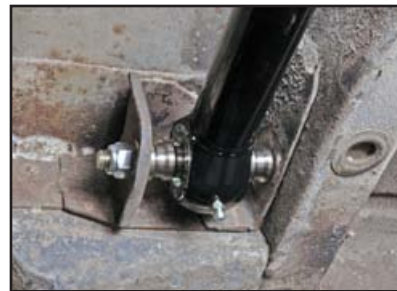
Lower links mount at OEM leaf-spring brackets.
