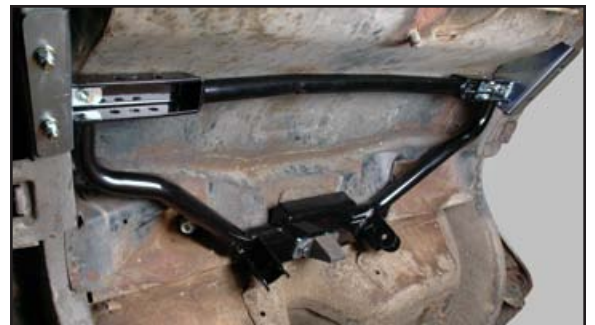
"Self-positioning" system utilizes existing pinion snubber and top shock mount factory bolt holes.
