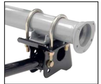
g-Bar axle bracket assembly.
